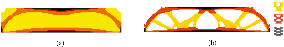
Fig. 16. The regularized design region for MBB structure and the optimal results obtained by the proposed method.
